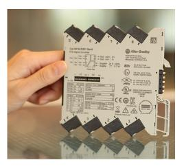
Instead of running expensive cable to the control system (for example, thermocouples for temperature), Analog Signal Conditioners can isolate and convert to a high-level signal that is easier to transmit (for example, 4...20 mA).
